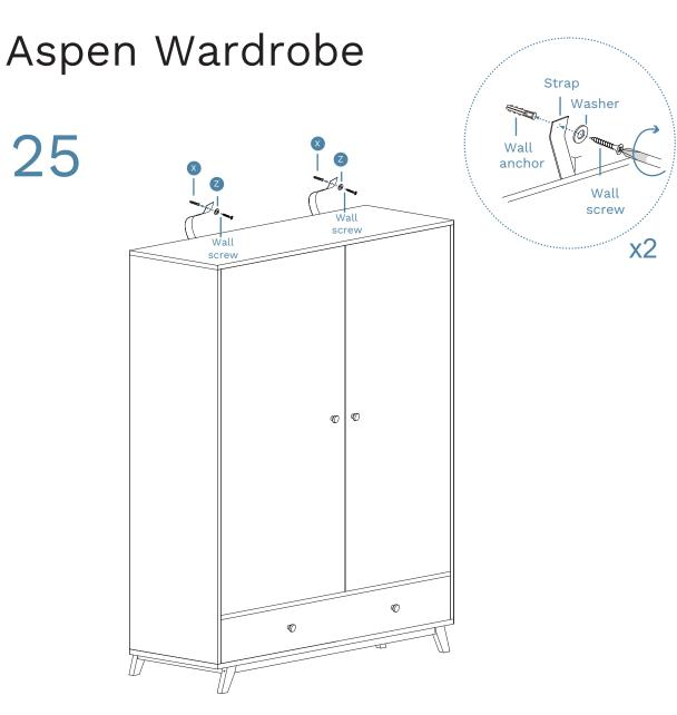
Once assembled lift furniture into place, do not drag. Use a drill to create a small hole lining up with the top of the safety stap (W). Fasten to wall using wall anchor (X), washer (Z) and screw. Ensure the unit is balaced and steady before use. You're done, enjoy!
