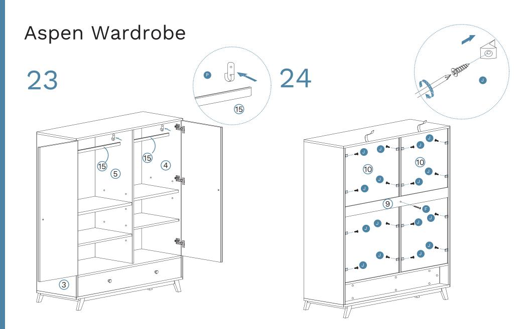
Attached panels [15] to clothes hager supports (P) as shown.Insert 16 x
